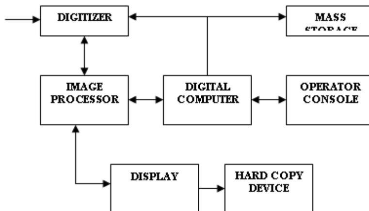
Fig 1 Block Diagram For Image Processing System
